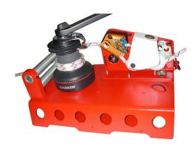
For decending and ropeing up with a fibre rope. The best working areas for fibre rope rescueing are steep or overhanging rock, steep forrest or lawn-areas, gorges and canyons. The optimum working range is up to about 100m at a working load of up to 250m. The best suited ropes are static fibre ropes with a diameter of 11 mm.
