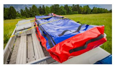
When fastening, it must be ensured that not only the transport bag alone, but also the stretcher in the interior is tensioned down. The transport bag serves exclusively to protect the stretcher during transport.
