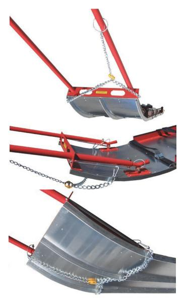
Very economic **flat-bottom rescue sled** for **one-man operation** on **easy to medium ski slopes**. Because of its flat bottom, the Canadier is designed to be operated in the fall-line.
