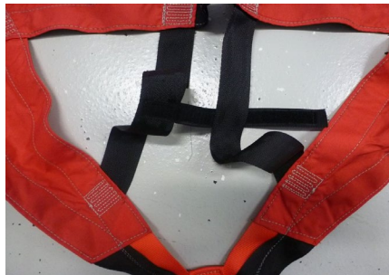
Fig. 10: Place the reinforcement strap under the right bottom belt
