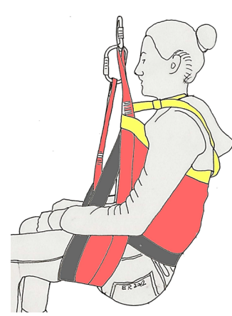
Fig. 17: 10 cm lengthening of crotch strap with a karabiner = slightly more upright position
