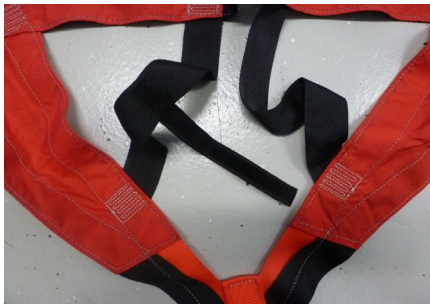
Fig. 9: Reinforcement strap sewn onto left bottom belt
